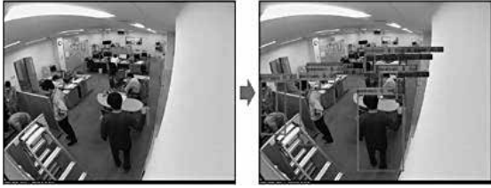
Figure 1. Examples of photos taken by Raspberry Pi Camera and detection results. Detection accuracy is high within a range of 6 to 8 meters from the camera. On the other hand, some cameras are less accurate for distant occupants.
